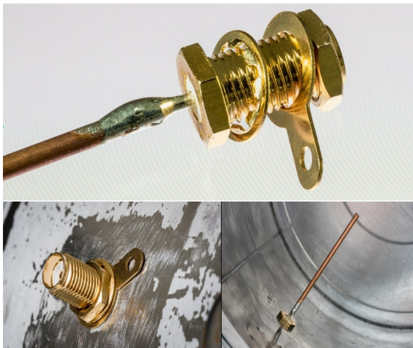
Figure 7. Installing the antenna element into the can
