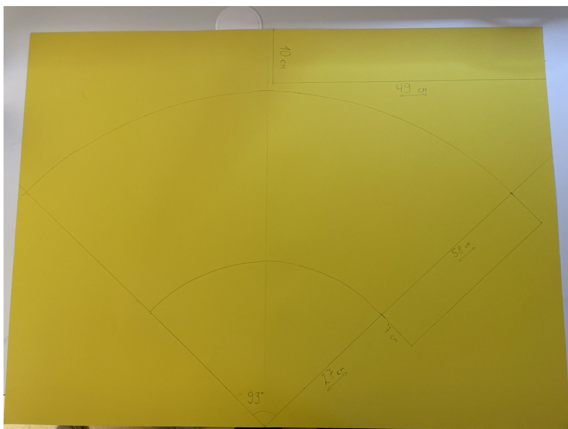
Figure 4. Marked elements before cutting
